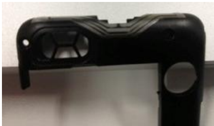
3D printed antenna with ForTii DSP82, Ag layer 4 \mu m, no Cu/N
