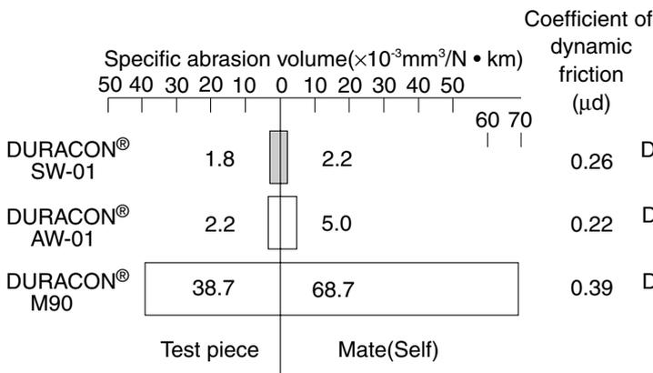
Fig. 1-9 Friction and Abrasion Characteristics Against DURANEX<sup>®</sup> 3300 (GF30% PBT)
