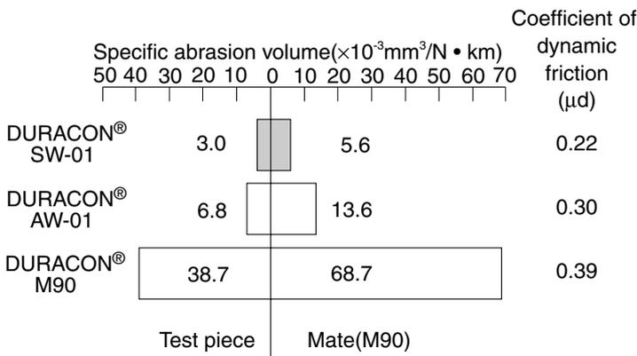
Fig. 1-7 Friction and Abrasion Characteristics Against S55C(Metal)
