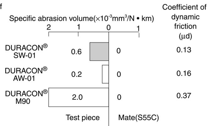
Fig. 1-8 Friction and Abrasion Characteristics Against Same Material
