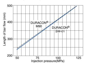
Fig. 3-1 Length of Bar Flow (2mmt)
