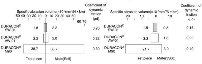
**SW-01** has rigidity comparable with that of M90, a general purpose grade **Duracon** despite of its improved sliding efficiency, so it is readily available for use in all applications now served by M90-44.
