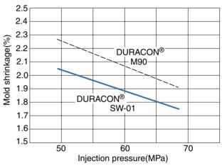
Molding conditions Cylinder temp. : 190-190-170-150°C Mold temp. : 80°C Injection speed : 25mm/s Molding cycle : Holding pressure 20s/cooling 10s Mold : 120sq.×2mmt flat plate, side gated 4w×2t
